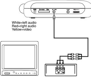
2 Plug the connectors on an optional RCA cable into the connectors on the other end of the supplied A/V cable. Make sure that the colors on the connectors match.
